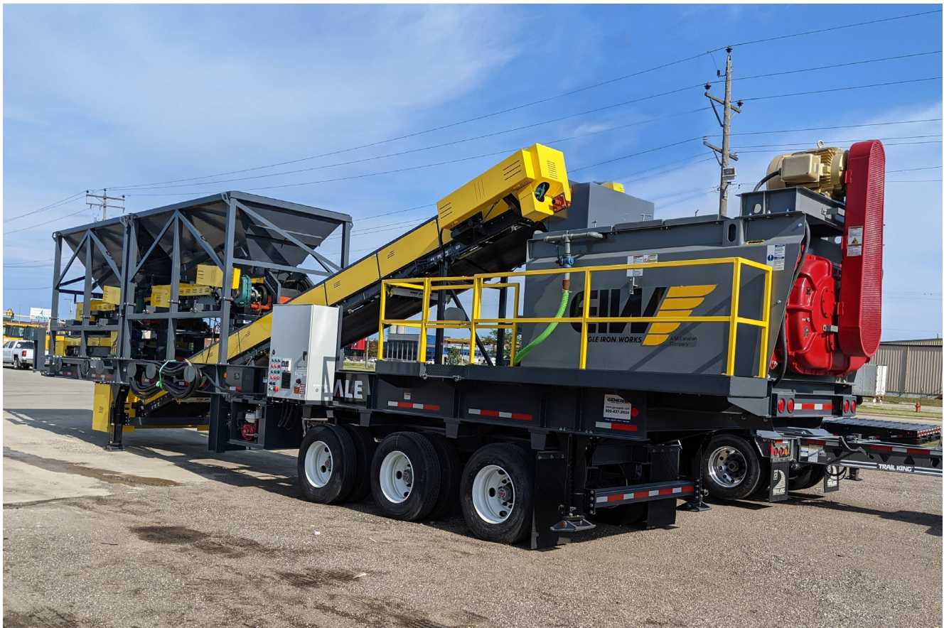
A portable EIW Pug Mill Mixer complete with a 2 hopper feed system
